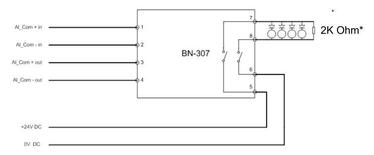
\* End-of-line resistance 2kohm, FAD circuit end-of-line monitoring
