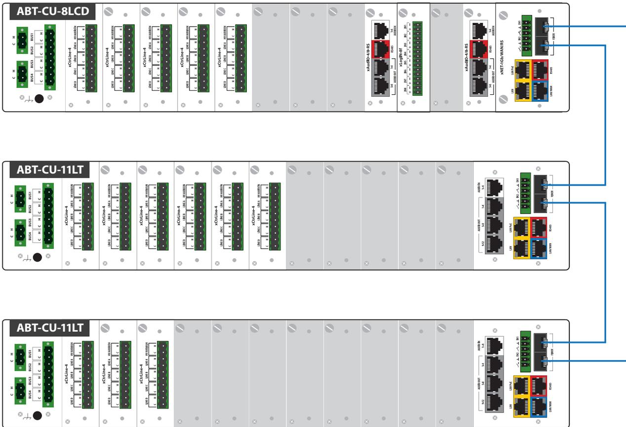
Drawing 65. RING topology control units connection (fiber connection)
