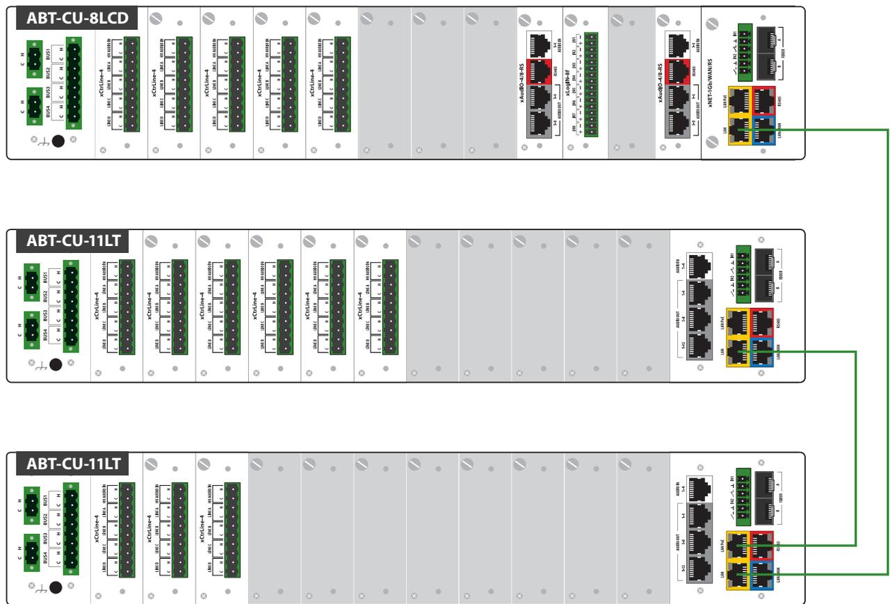
Drawing 64. Example of daisy chain topology control units connection
