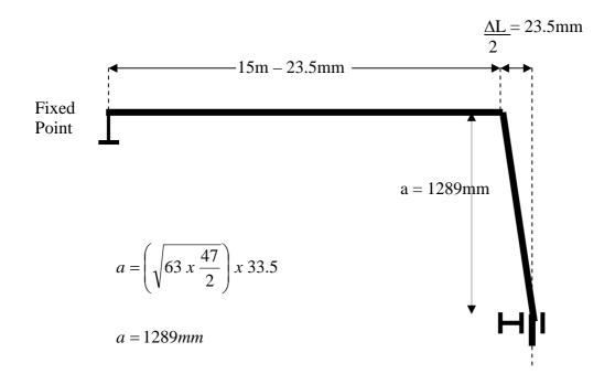
By pre-stressing the flexible arm it has been possible to reduce the arm length, and the pipe can now expand and allow (a) the flexible arm to straighten and to relieve the pre-stress.
