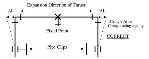
The bracket has been placed to ensure even distribution of length change, either side of the fixed point. It is not advisable to place the bracket so that the distribution is uneven.
