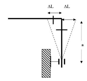
To calculate the length of a flexible arm (a) the following formula can be used.
