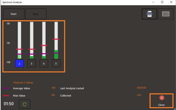
It is recommended this test be run within various different areas of the installation for better results. For every different area the timer should be reset, and the procedure should run again for at least 1 minute. This process should be repeated until the entire area of a wireless network is covered.
