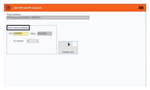
The user can configure the SID and RF channel of the gateway in order to change the network of the device. The initial network of a new, unconfigured gateway is the default network and it is recommended that the user assign the device to a different local network.
