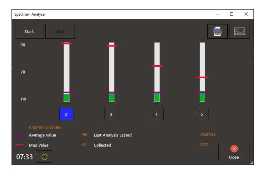
Let the procedure run for at least one minute (according to the timer bottom left). It is recommended to run the test into many areas of the installation for better results, reset the timer on each new position and count at **least 1 minute of scanning**, until you cover the area of a wireless network. In areas that another independent wireless network will be installed, run a new measurement by stopping the previous first.
